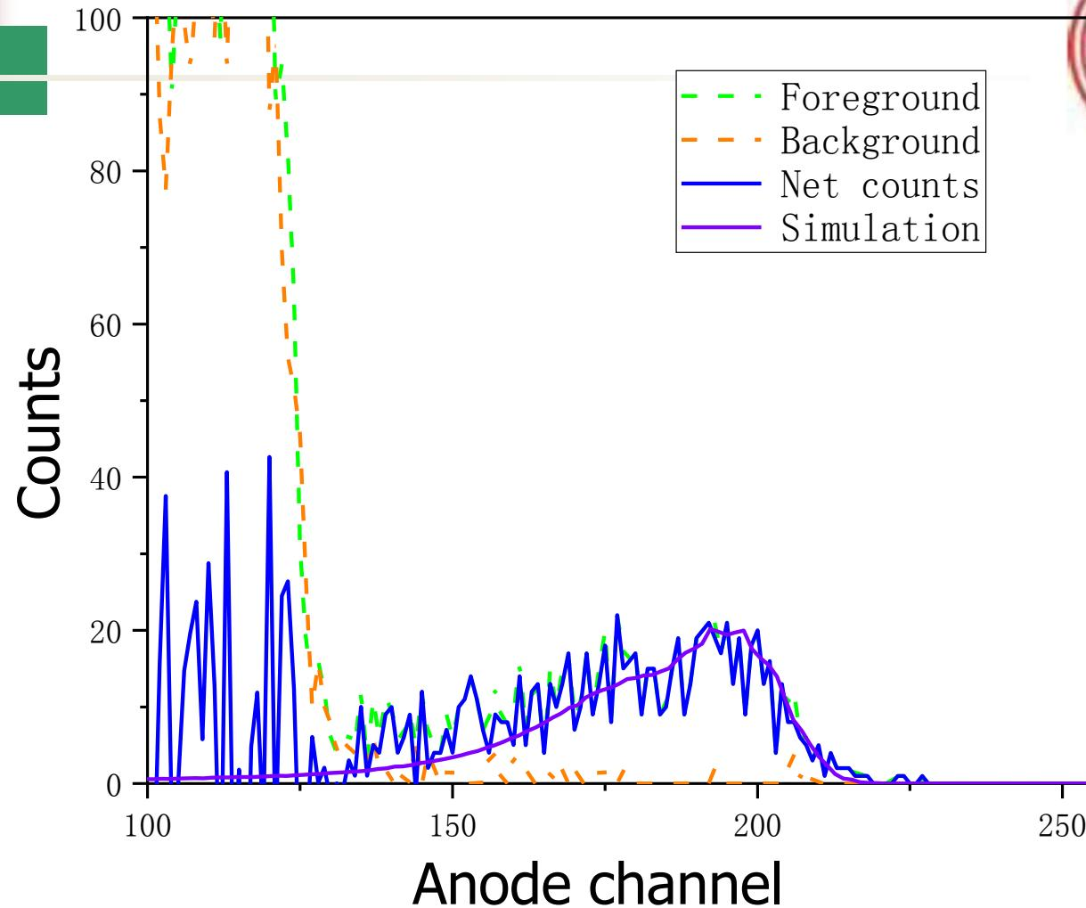
Anode spectrum of the  $^{144}\text{Sm}(n, \alpha)^{141}\text{Nd}$  reaction
