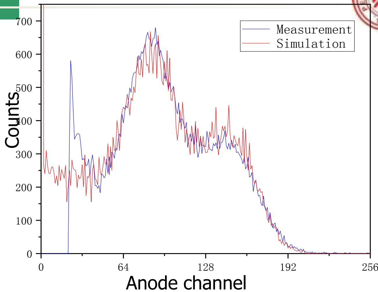
Anode spectrum of the  $^{238}\text{U}$  fission fragments at  $\text{En} = 5.5 \text{ MeV}$
