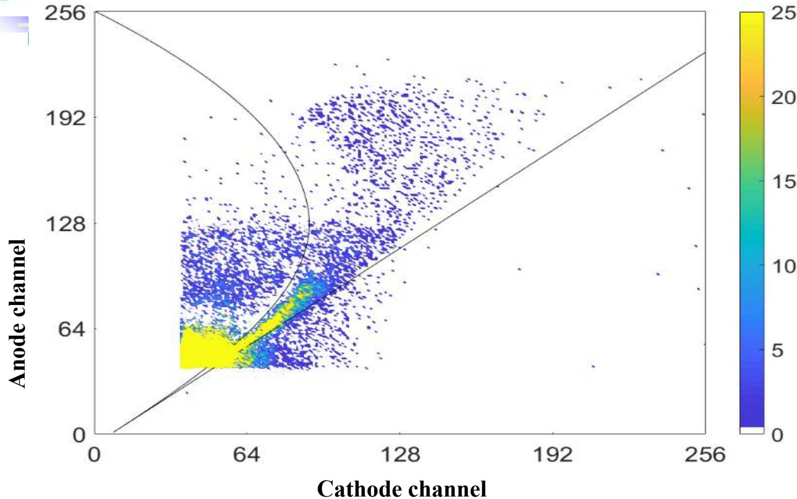
Two-dimensional spectrum of the  $^{144}\text{Sm}(n, \alpha)^{141}\text{Nd}$  reaction at  $E_n = 5.5 \text{ MeV}$  in the forward direction
