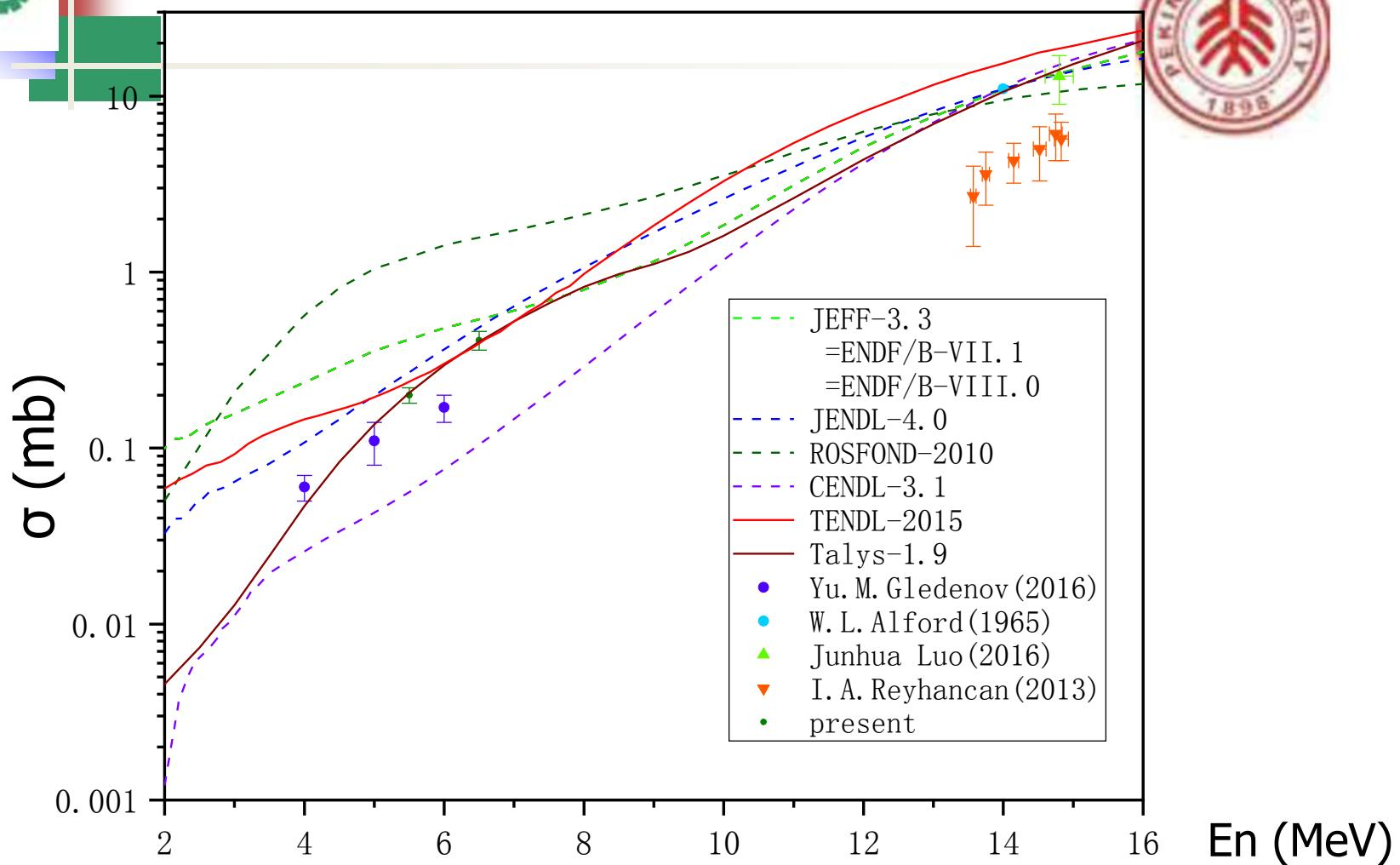
Present cross sections of the  $^{144}\text{Sm}(n, \alpha)^{141}\text{Nd}$  reaction compared with existing measurements, evaluations and Talys-1.9 calculations
